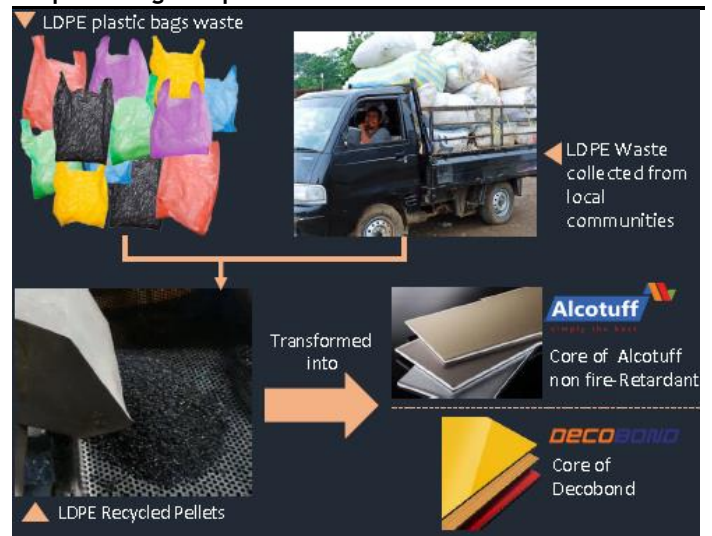
Fig 29: Recycled LDPE plastic bags are used as the core layer for producing ACP panels
