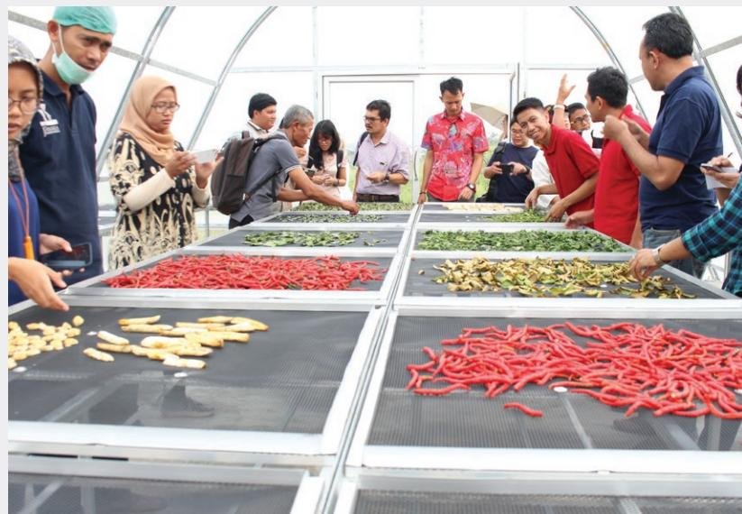
Drying Process of Agricultural Products Using Solar Dryer Dome ▲
